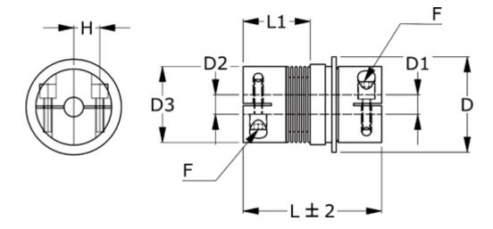
D = 94Nom. torque NM (Tkn) = 80NM overload torque range 2 D1 = 30Position engagement = C = Synchronous
